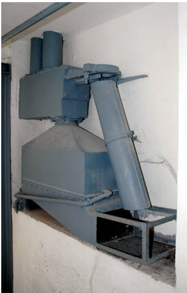
A Degesch hot air fumigation device. At the top the can opener controlled from the outside. The Zyklon pellets slide through the pipe into a wiremesh basket at the bottom, through which warm air is conducted by the heater/fan unit (below the can opener).
